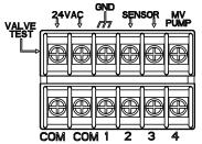
VALVE TEST – Use this terminal to test a value for proper function.
