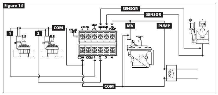
Step 1 – Route valve wires from the valves, master valves, pump relay and/or sensor into the controller cabinet.
